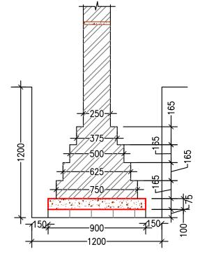
SECTIONAL DETAILS OF FOUNDATION (250MM THK. WALL)
